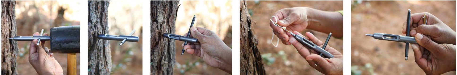
Microcore sampling using Trephor tool (Rossi 2009)
