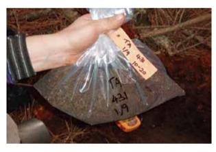
8) When finished sampling put a clearly marked label inside the bag and tie another label around the top of the bag.
