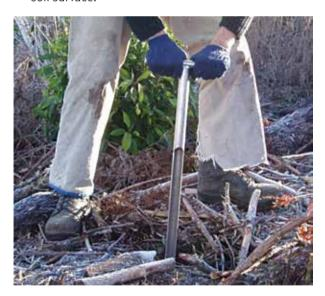
3) Push the Hoffer tube into the ground 10 cm or the sampling depth required and carefully pull out again.
