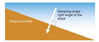
Place the Hoffer tube at right angles to the mineral soil surface.
